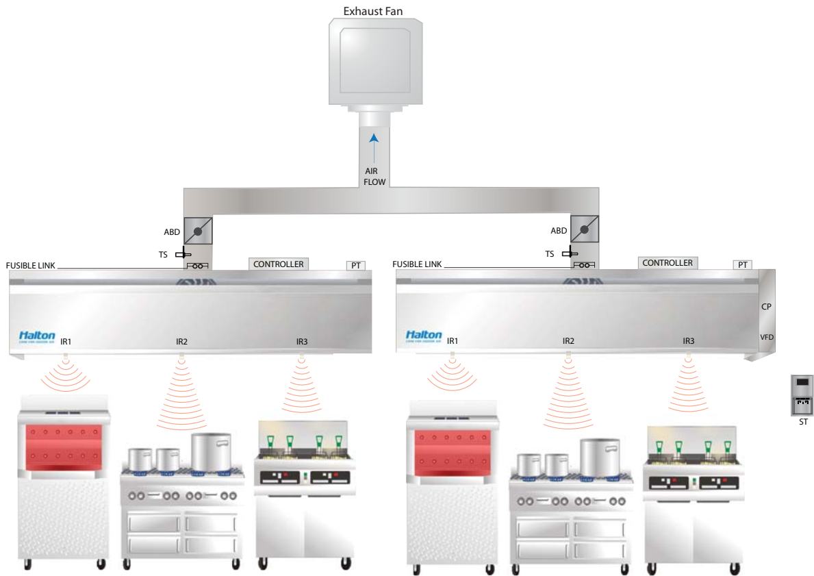
Figure 2: Multiple Hood M.A.R.V.E.L. Installation
